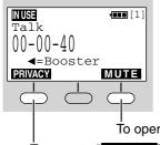
Three soft keys are used to select functions displayed directly above the keys. Functions displayed above the keys will change depending on the state of use.
