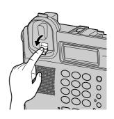
**2** Press the tabs in the direction of the arrows (①), then remove the wall mounting adaptor (②).
